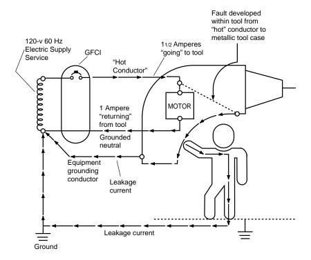
GFCI monitors the difference in current flowing into the "hot" and out to the grounded neutral conductors. The difference  $\binom{1}{2}$  ampere in this case) will flow back through any available path, such as the equipment grounding conductor, and through a person holding the tool, if the person is in contact with a grounded object.
