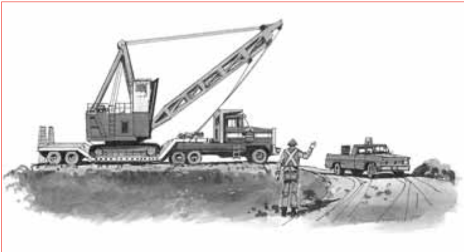
The boom of the grapple yarder has been lowered for transport.
