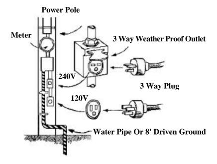
Make sure that electrical power tools have a true ground or are double-insulated. For example a drill has a third wire which is the ground wire. This means that the current will follow the ground wire—not the operator. If a drill develops a short, have it repaired before using it again.
