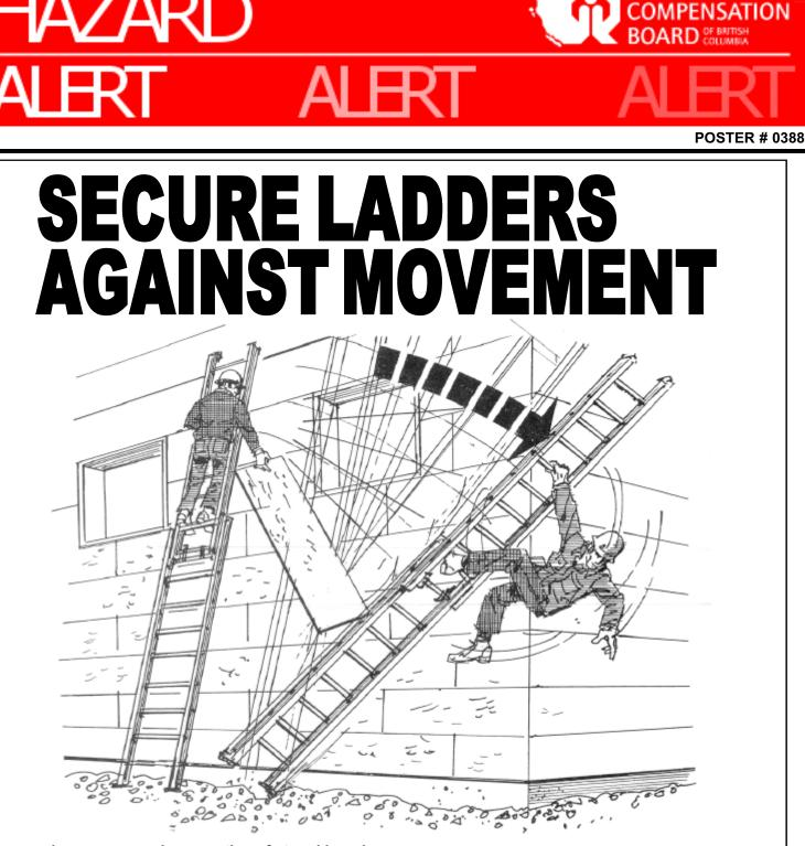
Two workers were carrying a section of strand board while climbing two separate ladders when one of the ladders slid sideways and the worker fell approximately 10 feet to the ground. The worker landed on his head and right shoulder, and he later died from severe head injuries suffered in the fall. Whenever you are climbing a portable ladder, be certain that all four ends are secured against movement. Do not carry any heavy or bulky object while climbing up or down a ladder.
