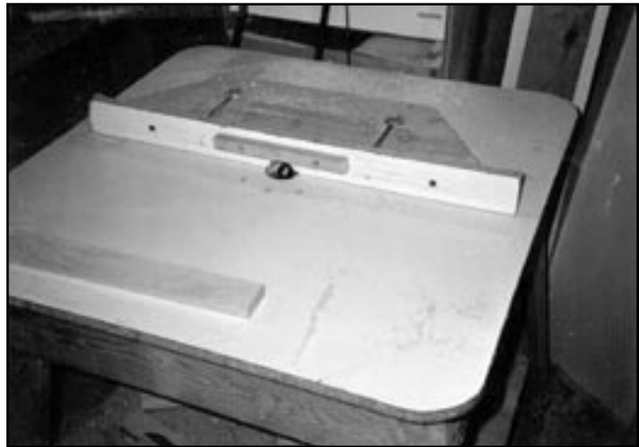
Exposed cutting head on shaper
