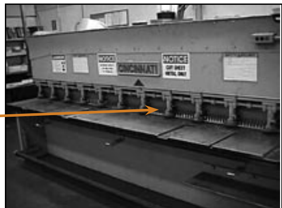
Unguarded hold-down devices on a power squaring shear.
