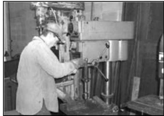
The stock can spin if not adequately secured to the table.
