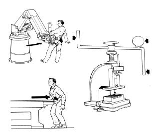
The diagrams below show **transverse motion hazards** with various machinery parts and equipment: at conveyor belt, band saw, belt sander, lift truck, robots, drill press, press, etc.
