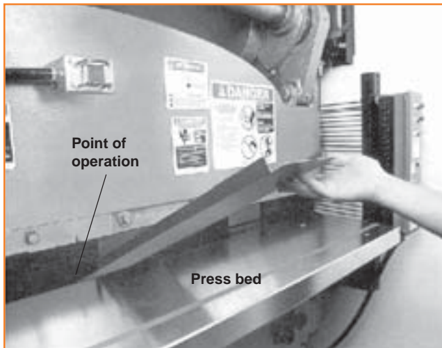
Figure 25. Power Press Brake Bending Metal
