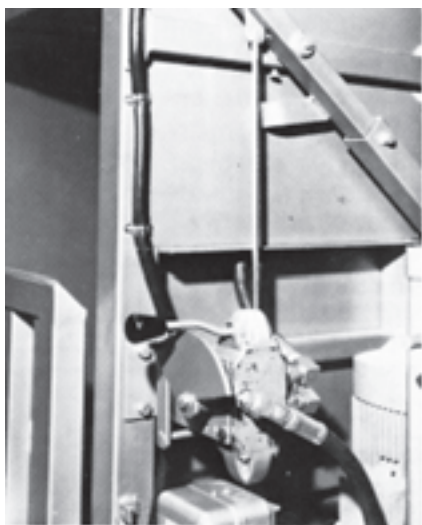
Fig. 6: Mechanical interlock (guard open)
