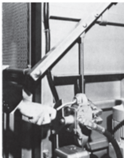
Fig. 7: Mechanical interlock (guard closed)
