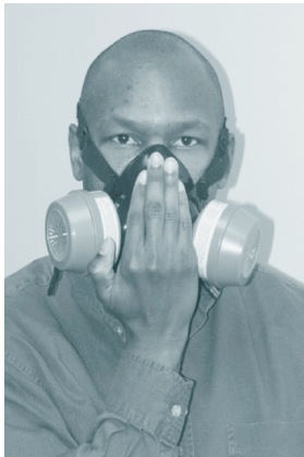
Positive-pressure seal check
