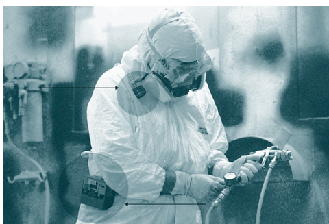
Personal air pump and sampling media used to measure air contaminants during spray painting
