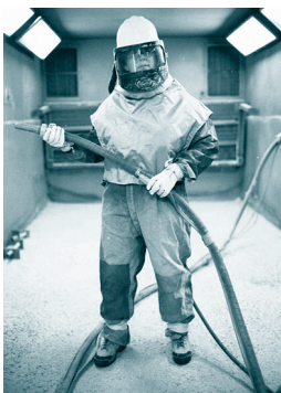
Supplied-air respirator (abrasive blasting helmet)
